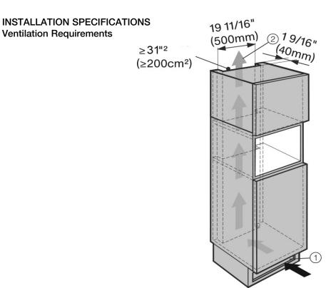
Air intake  $\ \, \mathbb O \$  occurs via the plinth at the bottom of the appliance and the air escapes at the top  $\ \, \mathbb O \$  at the rear of the surrounding cabinets.
